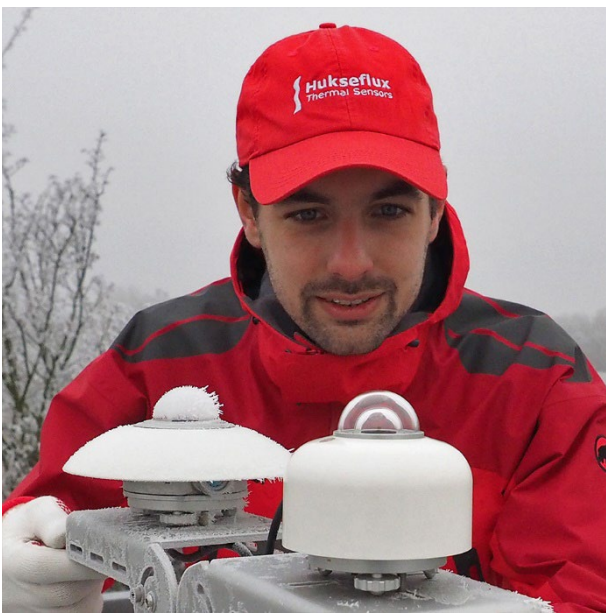
Figure 5 Heating counters frost and dew deposition: clear difference between a heated and non-heated pyranometer.
