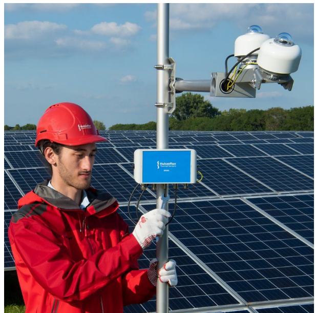
Figure 7 Two SR300-D1 pyranometers that are connected to the SPD01 Surge Protection Device. With the optional SPD01, you can upgrade surge immunity to Level 4.
