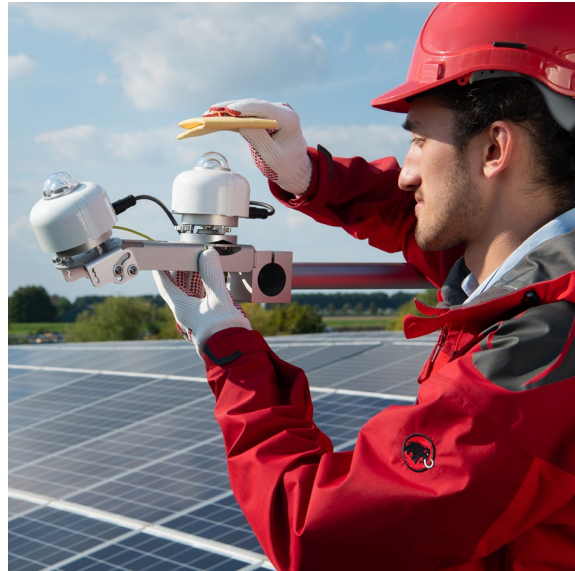
Figure 0.6 SR300-D1 includes a digital tilt angle measurement, very practical for remote checks of instrument orientation. The image shows two SR300-D1's in PV system monitoring, one measuring in Plane of Array (POA).
