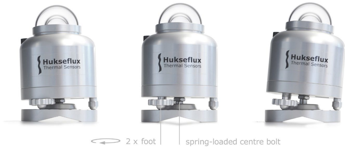
Figure 0.9 LM01 levelling mount is the most popular option for pyranometers: practical spring-loaded mount for easy mounting, levelling and instrument exchange on flat surfaces. The spring-loaded mounting has the advantage that levelling can be done quickly, without unlocking the instrument.
