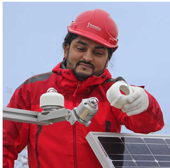
Figure 0.7 PMF series pyranometer mounting fixtures can be used for easy installation of pyranometers. On the left, PMF01 pyranometer mounting fixture with one SR30, and on the right PMF02 with two SR30 pyranometers. Both fixtures allow mounting in Plane of Array for PV system performance monitoring and meteorological applications.
