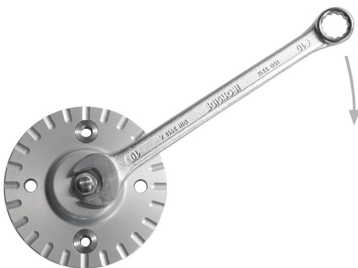
Figure 5.3.1.3 SR30-M2-D1 levelling mount seen from above: (un)locking with a 10 mm spanner
