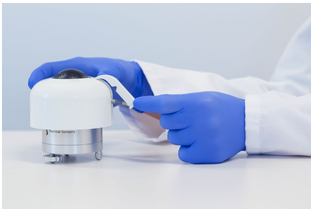
Figure 4 Pyranometer model SR30, with DP01 and sunscreen.
