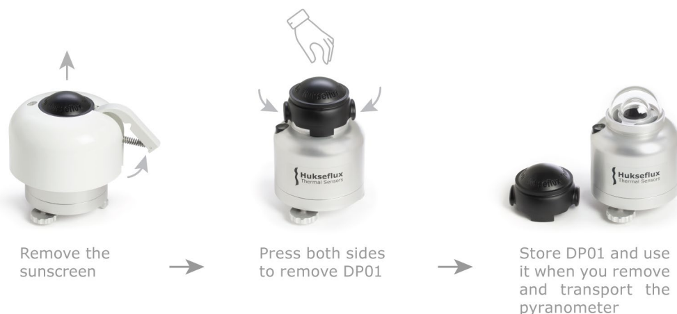
Figure 2 Removal of sunscreen and DP01.
