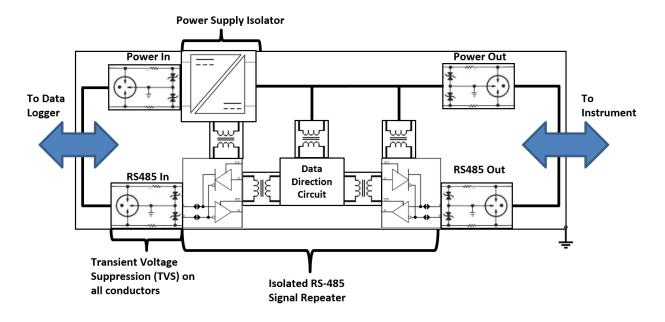
In the block diagram above, the "in" side (To Data Logger / DAS) features an isolated 9-36 VDC DC-to-DC converter which provides an isolated 24 VDC supply signal to the "out" side of the SPD, to the pyranometer. This includes over/under voltage protection and reverse polarity protection. All other components implement an isolated auto-direction detecting RS-485 repeater between both "in" and "out" sides of the SPD device.
