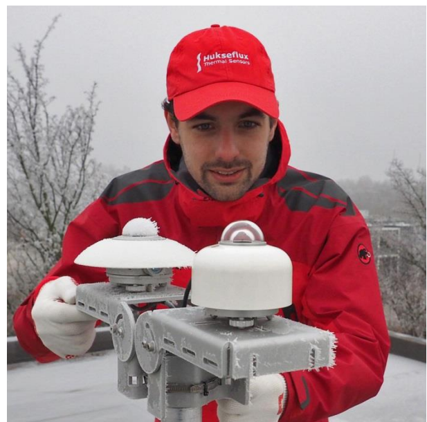
Figure 1 frost and dew deposition: clear difference between a non-heated pyranometer (back) and SR30 with RVH™ - Recirculating Ventilation and Heating - technology (front)
