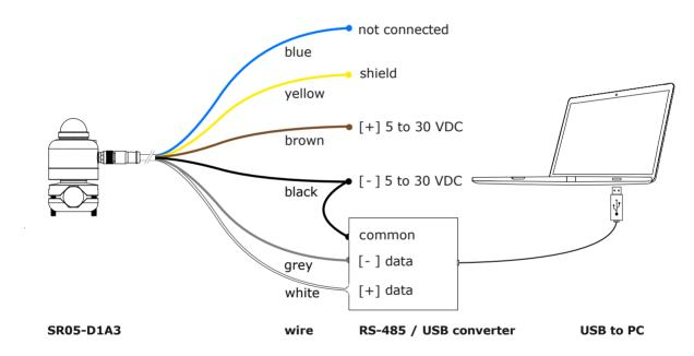
Figure 5.12.1.1 Connecting SR05-D1A3 to an RS-485 to USB converter and a PC
