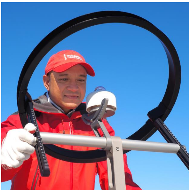
Figure 2 installation of the compact SHR02 shadow ring and a Hukseflux pyranometer is easy. When combined, a diffusometer is created, in which the shaded pyranometer measures diffuse radiation only.
