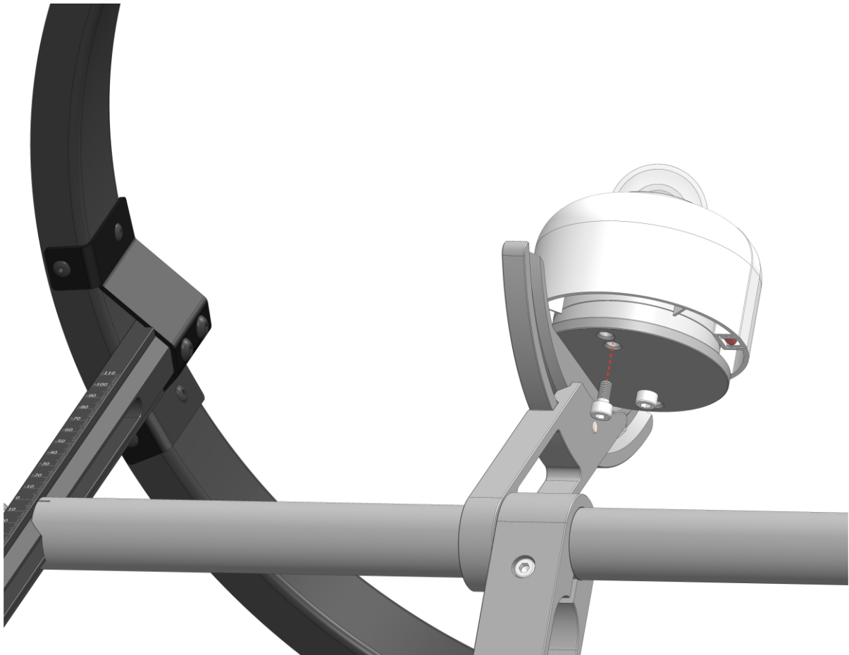
Figure 5.4.3.1.1 Mounting an SR15 pyranometer on SHR02
