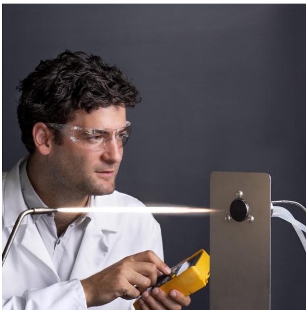
Figure 2 HFS01 is the sensor of choice for studies of concentrated sun and high-intensity flames
