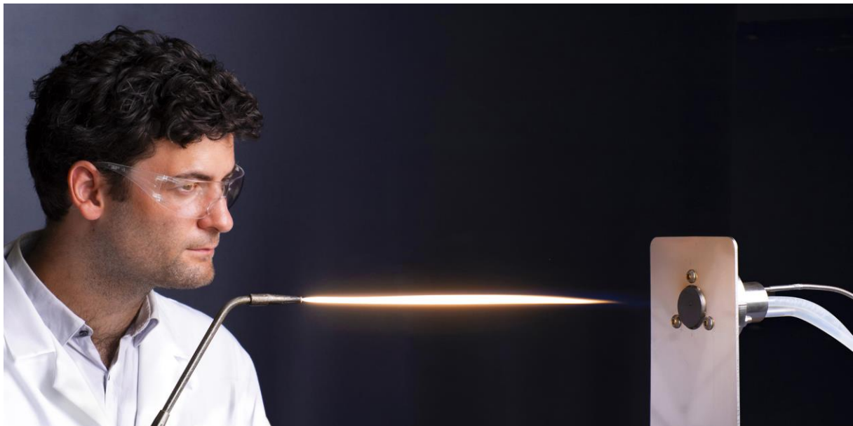
Figure 0.2 HFS01 is the sensor of choice for concentrated sun and high-intensity flames
