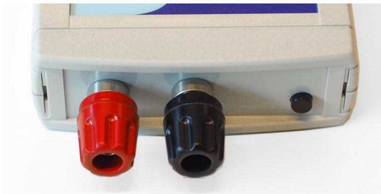
Figure 4.1.1 Connectors and on/off switch on LI19. Connectors are 2 x female chassis plugs for 4 mm banana plug, with screwed signal wire clamps
