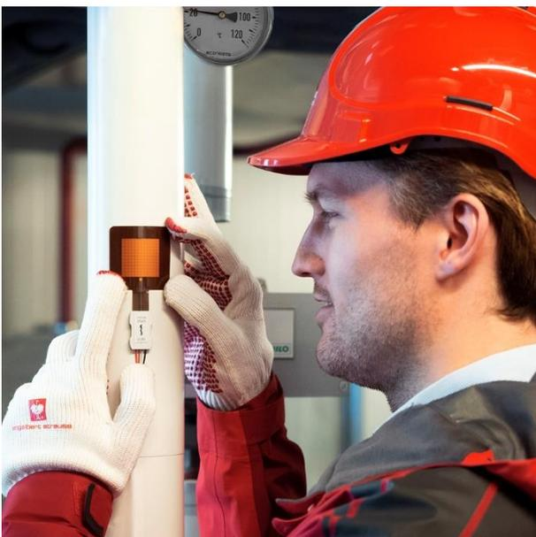
**Figure 2** FHF04 being installed to measure heat flux on a pipe
