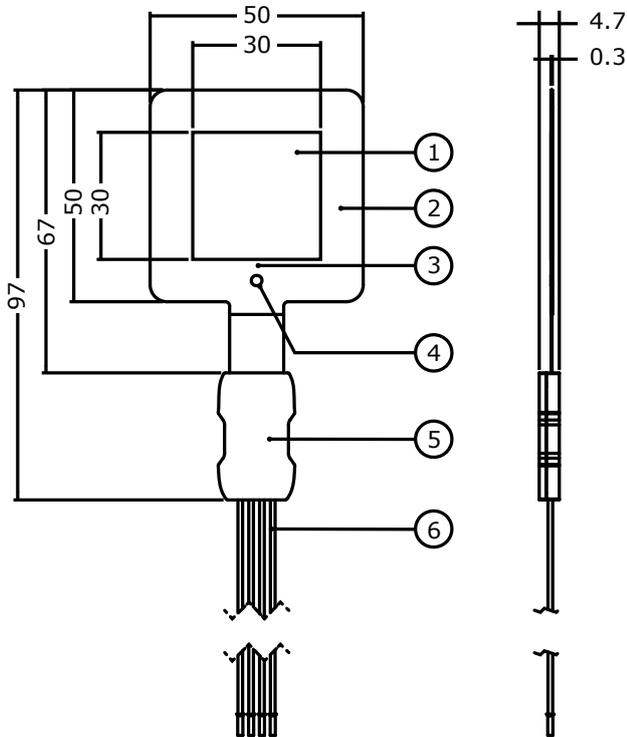
**Figure 4** FHF04 heat flux sensor: (1) sensing area with thermal spreaders, (2) passive guard, (3) type T thermocouple, (4) dot indicating front side, (5) metal connection block showing serial number and sensitivity, (6) wires, standard length is 2 m. Dimensions in  $\times 10^{-3}$  m.
