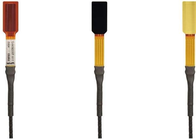
Figure 0.3 FHF03: with BLK-3015 and GLD-3015 stickers to measure radiative and convective heat fluxes separately
