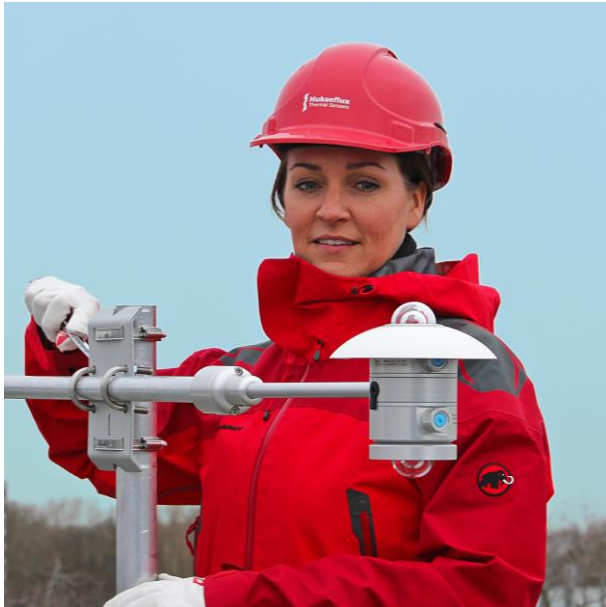
Figure 4 an albedometer being installed with its rod mounted securely to a mast thanks to ALF01 levelling fixture and CMF01 crossarm mounting fixture
