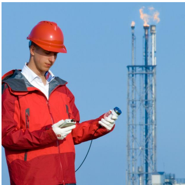
Figure 2 We offer an extensive range of products for fire testing and studies of flares. The picture shows HF03-LI19 portable heat flux sensor with read-out unit.
