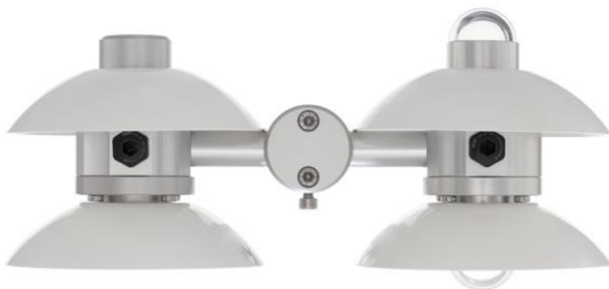
Figure 1 NR01 4-component net radiometer, including two pyranometers, two pyrgeometers, a heater and a 2-axis levelling assembly
